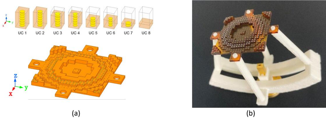
Fig. 1: 3D printed metamaterial transmitarray: (a) 3-bit metamaterial unit cells (UCs) and the 3D model of transmitarray, (b) Photo of the prototype.
